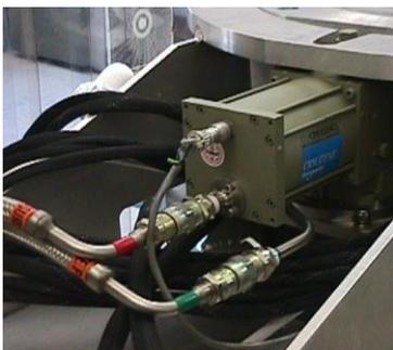
Example of an Installed Cold-Head.
